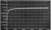
current or insulation resistance as a function of time as an X-Y graph or
