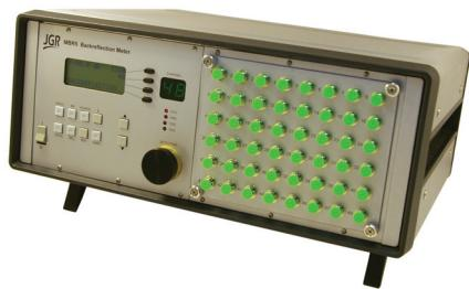
The MBR5 Multi-Output Backreflection Meter is an instrument developed with extremely stable optics for precise measurement of backreflection, insertion loss and power. Available with 4, 12, 24, or 48 output channels, the MBR5 is a practical choice for both single fiber and ribbon fiber testing. The MBR5 features up to four built-in laser sources at wavelengths of 850, 1310, 1490, 1550 and 1625 nm (depending on fiber type), and can be configured for single-mode or multimode measurement.
