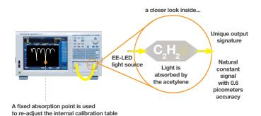
Ambient temperature change, vibrations and shocks affect the measurement accuracy of high precision instruments. We want our OSAs to be able to deliver always the precise measurements they were designed for, therefore our instruments are equipped with a light source for calibration. Calibration process is fully automatic and takes only 2 minutes to complete. It includes:
