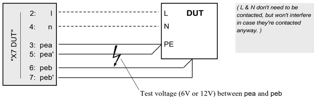
Or, using a connection panel (A3) and a test probe:
