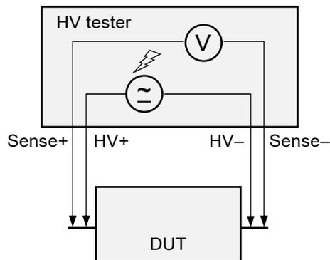
The "Sense Error" is triggered when a voltage of less than 90% of the set test voltage is measured back by the sense module. In this case, the measurement must be rated as invalid.
