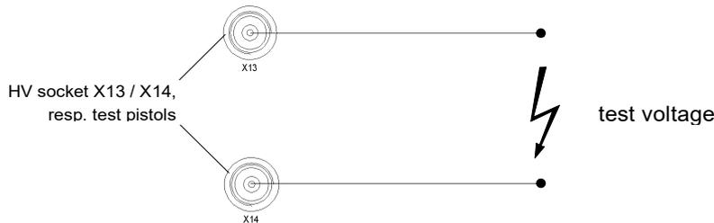
**Note:** With *Connection = Pistols*, there is no high voltage applied to X7 or connection box A3.
