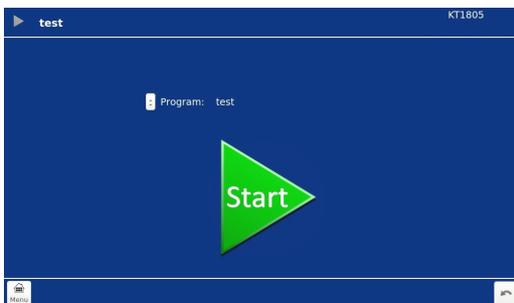
After the user-login, the device is showing the start screen with the latest used program active. You can immediately start testing by pushing the START triangle.
